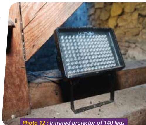
Photo 12 : Infrared projector of 140 leds of 3 mm (a widespread product).
