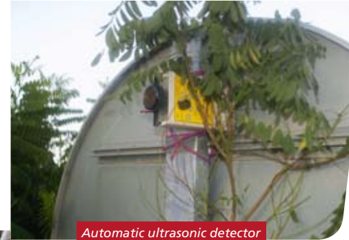
Automatic ultrasonic detector AnaBat™. © E. Cosson
